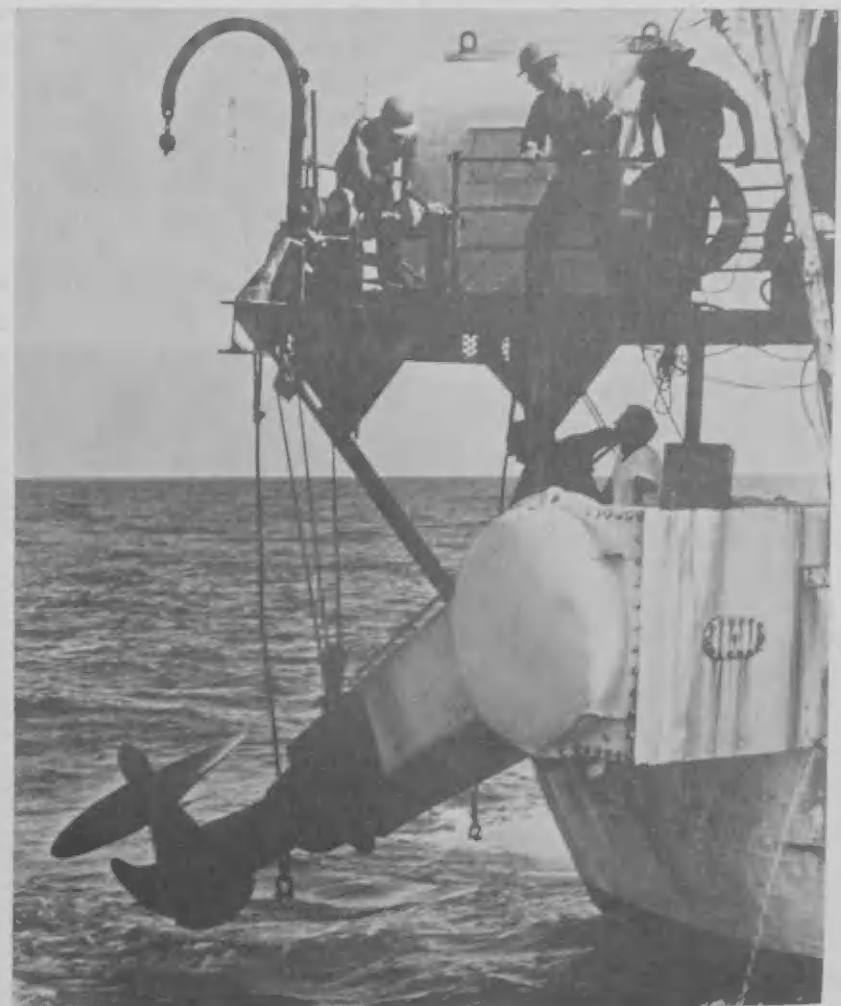
FOUR ELECTRICALLY driven propellers such as this one automatically correct for drift while the Caldrill I drills core holes in deepwater tests in the Gulf of Mexico.
